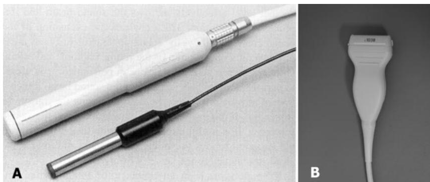
Figure 2. Typical transducers used with dedicated ocular ultrasound machines, **A**. A linear transducer commonly available on conventional ultrasound machines for lower-extremity duplex examinations and small parts scanning, **B**.
